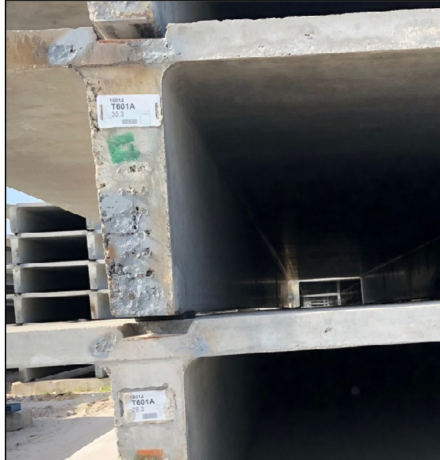
InfoSight Tag applied to precast concrete products
