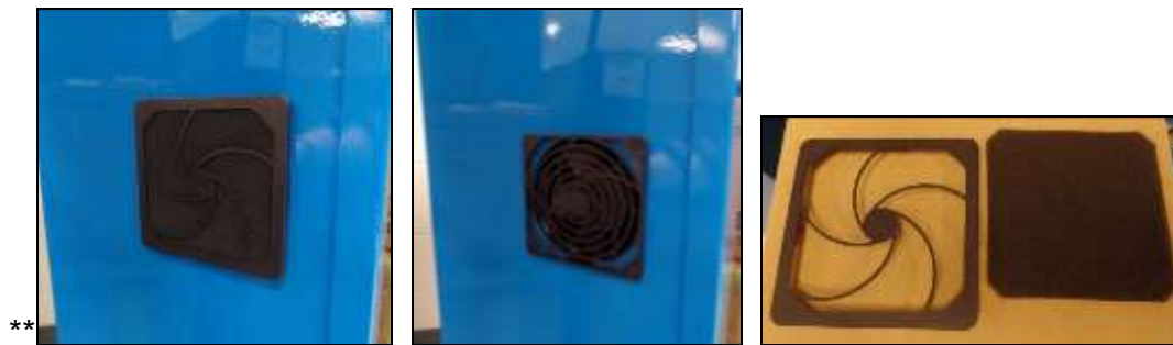
Figure 1 Side of LL28XX Printer shown with filter and cover in place (Left); with the filter and cover removed (Middle); and the filter and cover set aside (Right)
