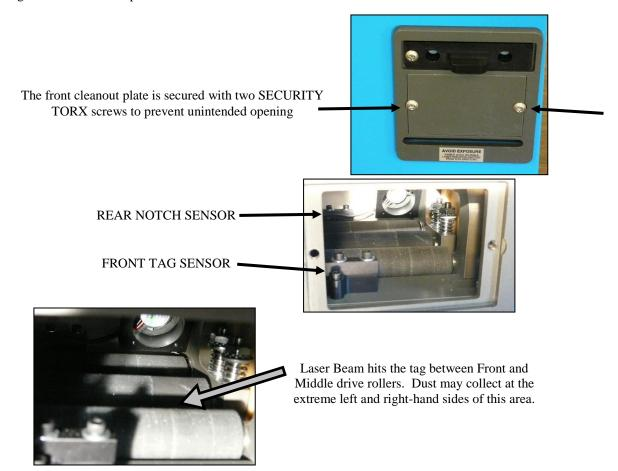
**CAUTION**: <u>ALWAYS</u> REPLACE THE FRONT CLEANOUT PLATE <u>BEFORE</u> CONNECTING POWER AND OPERATING THE PRINTER.
