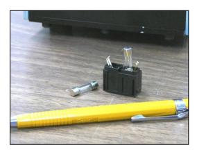
FUSES ARE RATED FOR 250V / 5A AC
