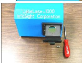
**CAUTION**: <u>DO NOT</u> TOUCH LENS WITH FINGERS OR ANY SUBSTANCE CONTAINING ALCOHOL, OR PERMANENT DAMAGE MAY RESULT.
