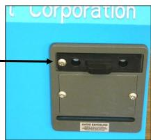
After removing the security screw, carefully open the slide to expose the lens.
