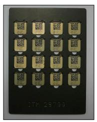
Left: This is an example of a multi-slot plate fixture for loading several small tags.
