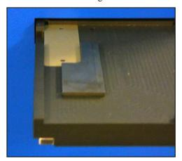
Left: A small single tag is loaded into the tag drawer. Notice the top left corner of the tag is aligned with the top left corner of the drawer. Also notice the "L" shaped tag shim aligned with the bottom right corner of the tag.
