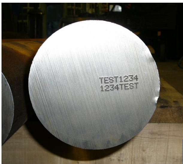
Typical stamped bar—1 of 8 in a gang
