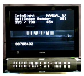
The OC code can sustain partial bar damage, linear damage through the entire length of the code, and spiral damage and remain readable. This significantly damaged code is STILL readable.
