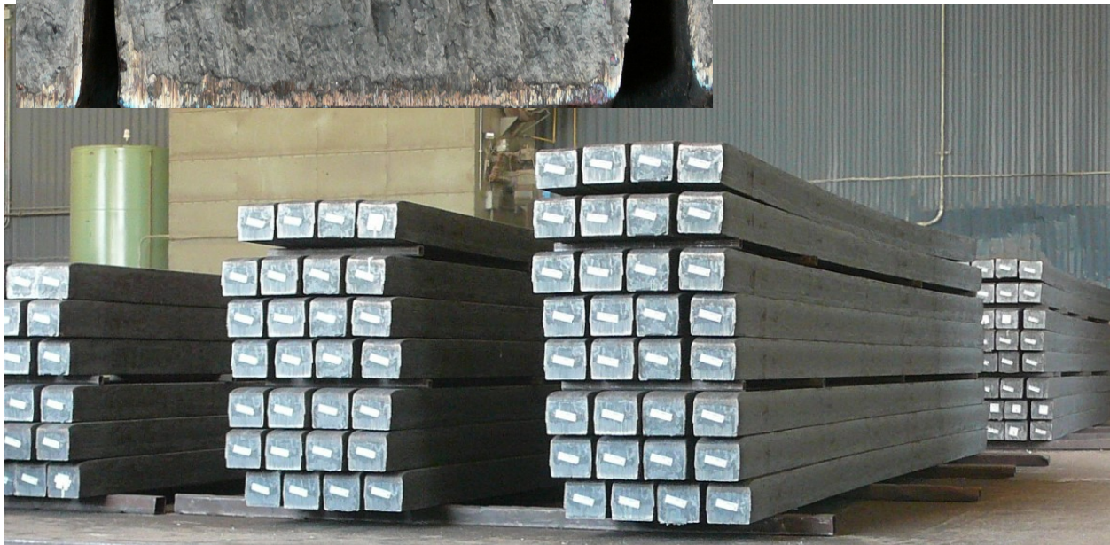
Below—stacks of bars with nailed-on tag ID
