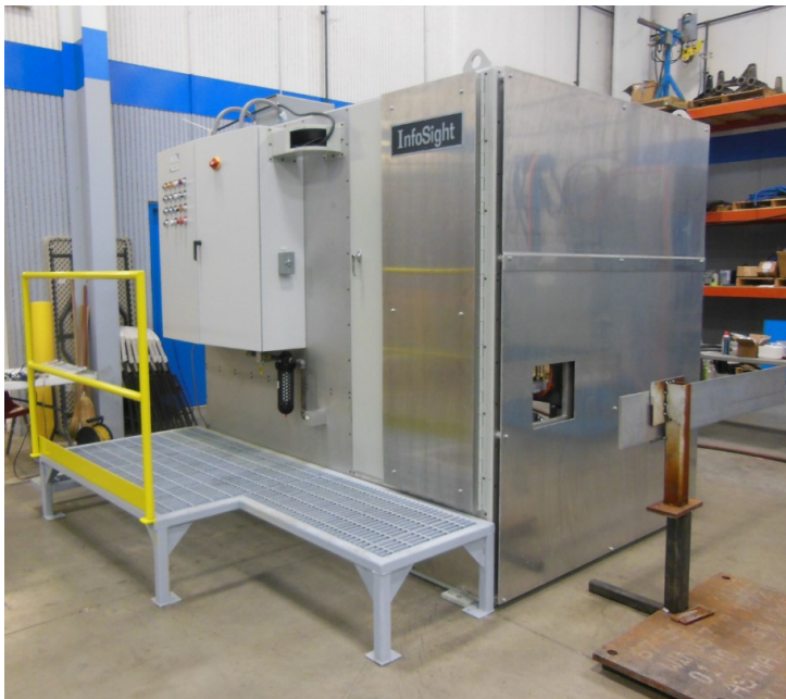
Tag nailer in testing in InfoSight shop
