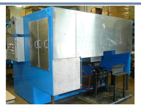
The InfoSight Model 2900 automatic single slab station tagging for stationary system slabs is the ideal bar code tag solution when it comes to MIG-welded tag identification of hot carbon steel slabs with high contrast marking.
