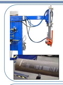
Automatic Stencil Marking Systems offer practical and cost effective alternatives to manual stenciling.
