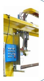
The X-Y Continuous Character Stencil Marking System automatically prints durable, high quality characters on cast shapes and coils.
