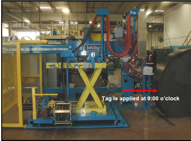
Examples of custom an automatic hot coil marking machines
