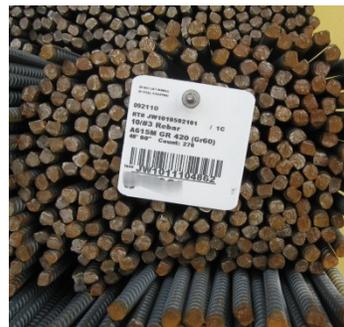
Individual long products (such as slabs) can also be either marked along their length or on the end face. Although each location has its advantages and disadvantages, the decision should be made based on downstream use of the identification (such as storage yard or reheat furnace entry line-of-sight accessibility). For bars, billets, blooms, etc. end face marking is preferred.
