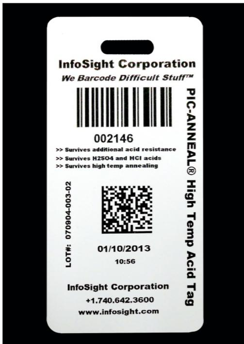
At the end of this time, InfoSight developed a tag that met Ivaco's needs – and would withstand the rigors put upon it by the processes of their different customers. Their PIC-ANNEAL® tag has a two-hour resistance to acid baths of 20% H<sub>2</sub>SO<sub>4</sub> at 180° F and 24% HCL at 100° F. It also withstands 1400° F heat for 48 hours and 1800° F for 2 hours.
