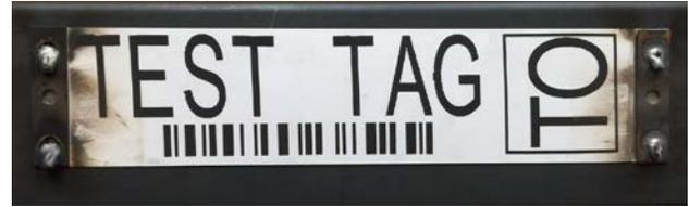
**Figure 10** - Tag with 3-mm preform attached by MIG welding.
