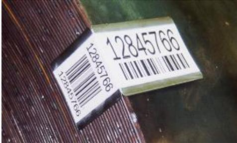
**Figure 9** - Folded tag attached to hot band coil by spot welding.
