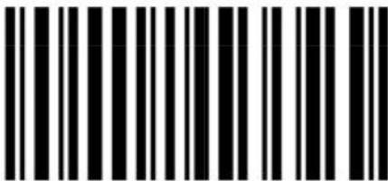
Figure 3 - Bar code with clean edges without voids
