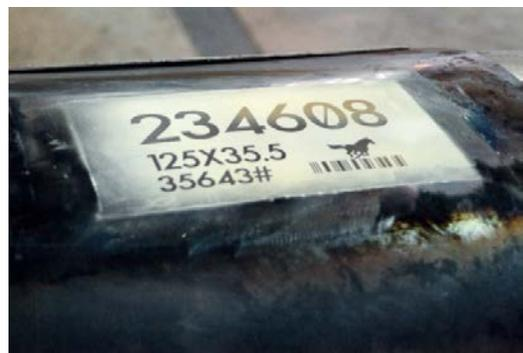
**Figure 11** - Direct marking with laser on white, sprayed patch on hot band.
