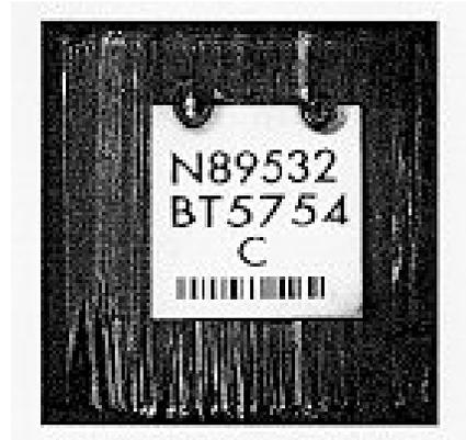
Figure 7 - Tag attached to billet end by plasma welding.
