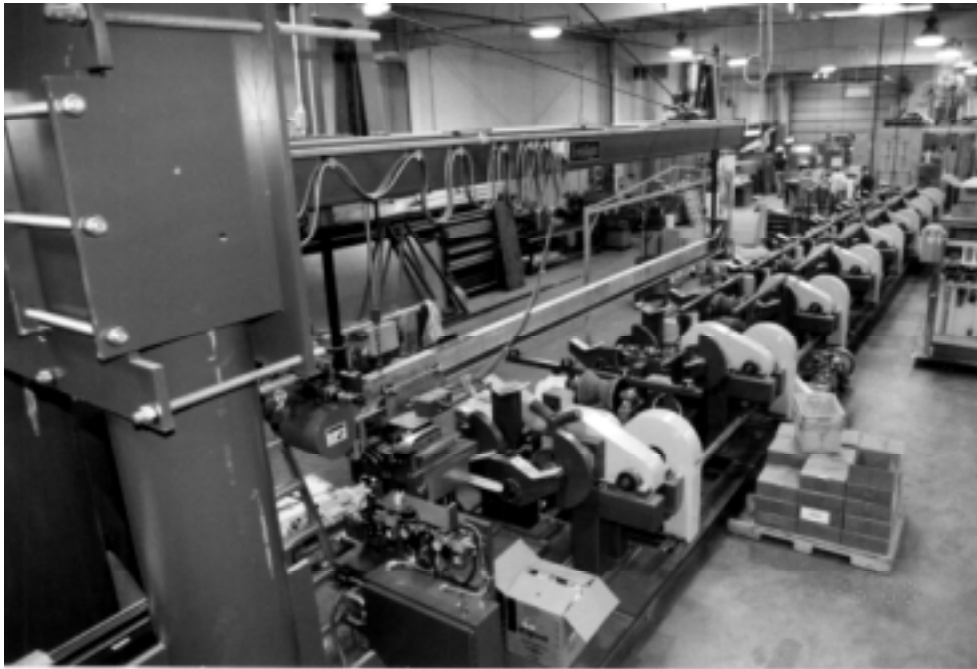
Figure 1 Cross transfer walking beam WMS system
