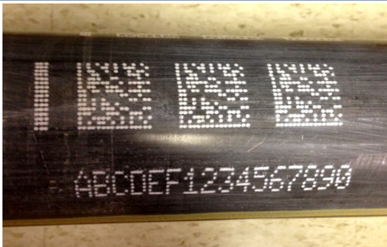
Typical redundant 2D Data Matrix bar codes on pipe—each approx. 1.25" (32mm)
