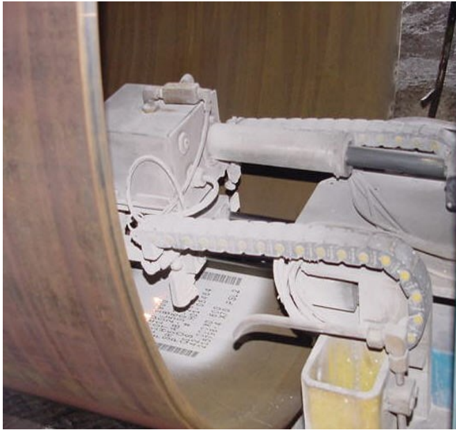
IDLMS System laser-marking the ID of a large pipe
