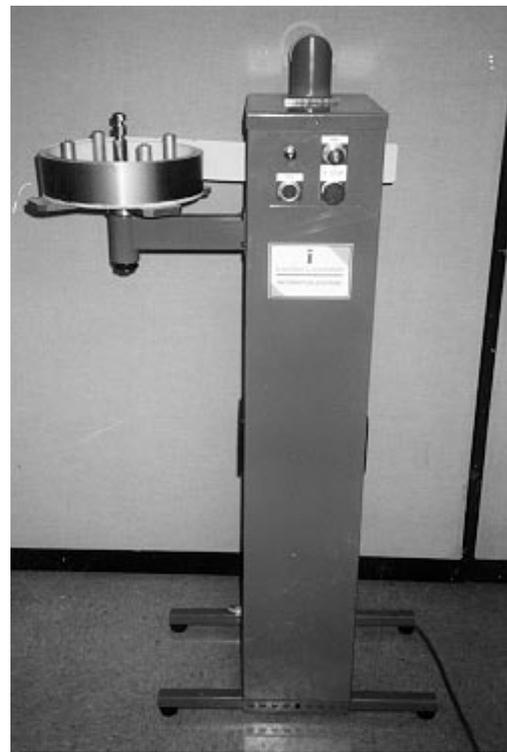
Fig. 5 — On-demand Laser Tag Printer
