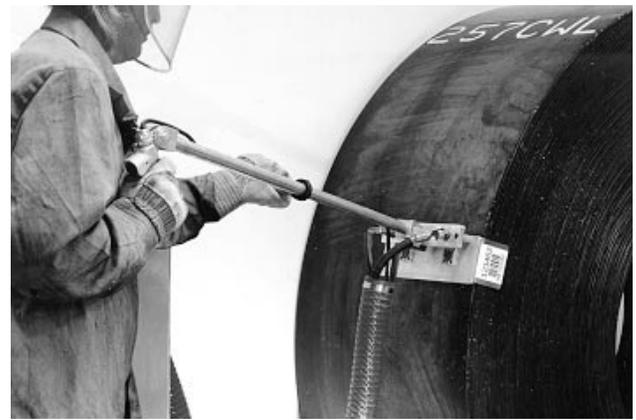
Fig. 4 — Tag application using a wand applicator
