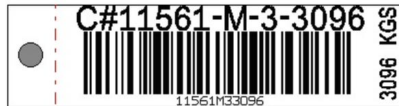
Figure 3- **Not recommended bar code** – HHHHH-alpha Q-S- WWW
