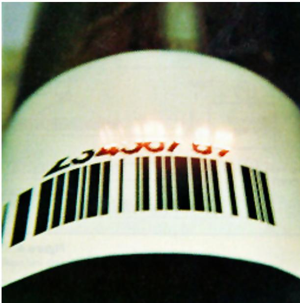
**Figure 2** - This tube has been laser-marked with standard bar code on its OD.
