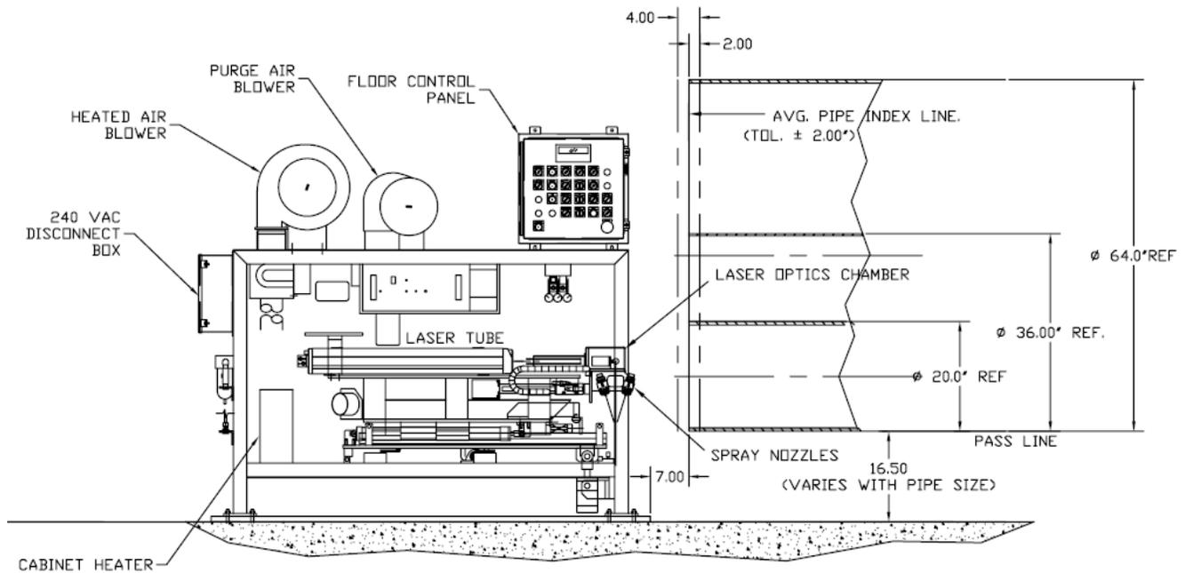
Figure 3 Typical IDLMS Marker Arrangement – side view
