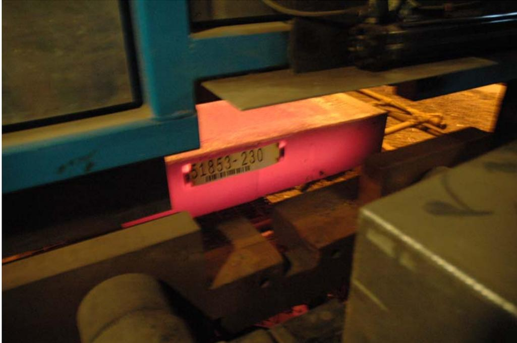
Figure 1 Typical Slab Tag after welding to the end of a torch-cut hot slab
