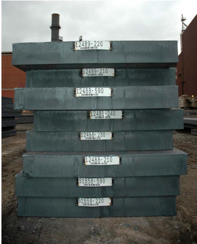
Figure 7 Typical stack of slabs in the storage yard
