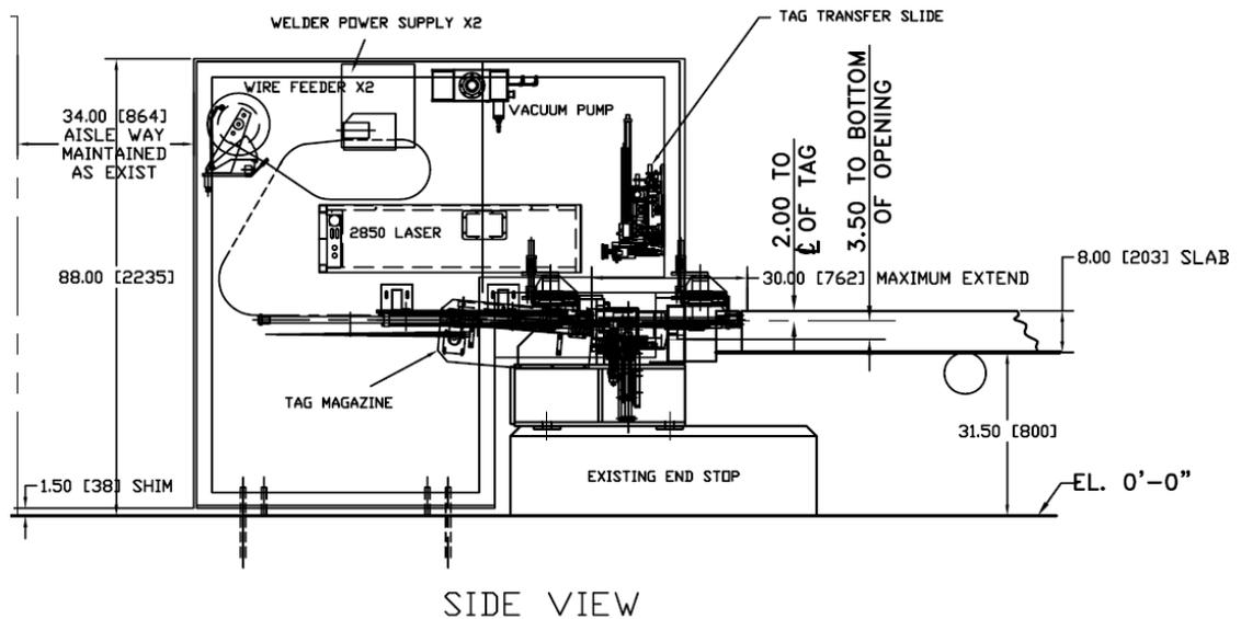
Figure 11 - SeverStal Slab Tagging Machine Arrangement – side view
