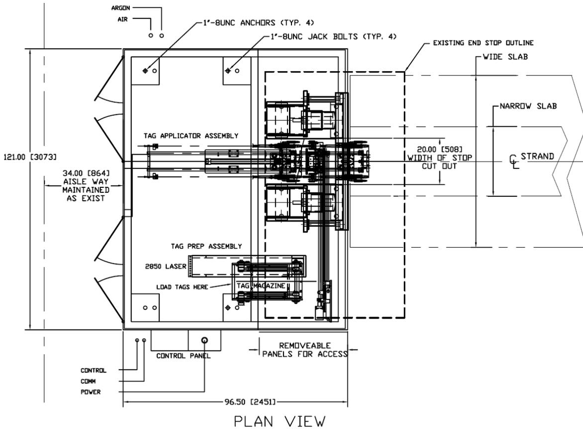
Figure 10 SeverStal Slab Tagging Machine Arrangement – plan view
