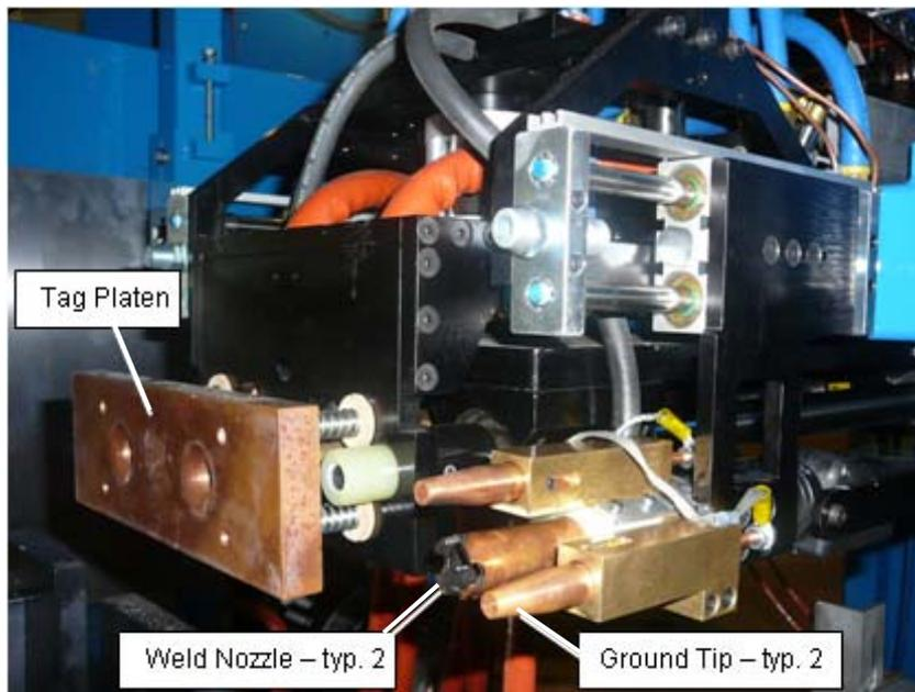
Figure 9 Close-up view of the Tag Applicator Assembly end tooling (heat shields removed)
