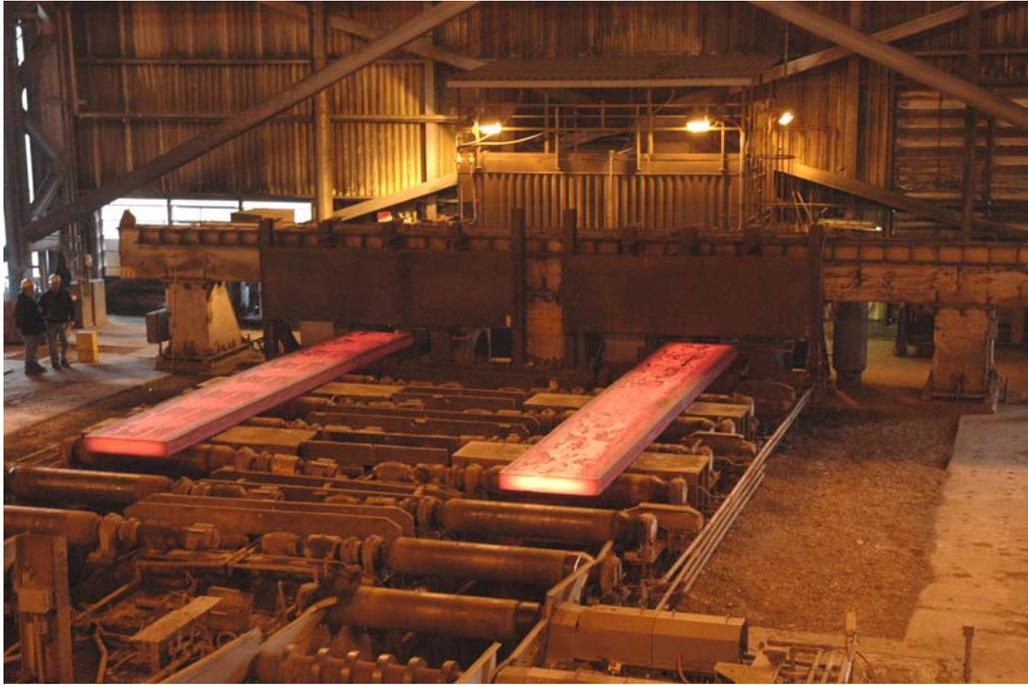
Figure 3 Slab Tagging Machines are located behind the end stops of Strand 2 (right) and Strand 1 (left)
