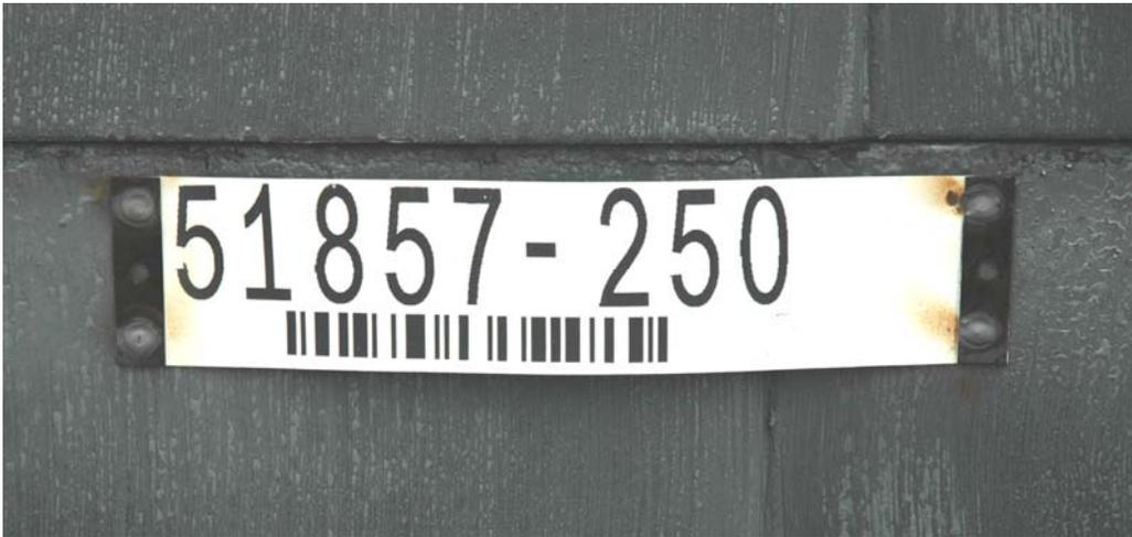
Figure 6 Typical Slab Tag welded onto a slab end with four corner MIG welds
