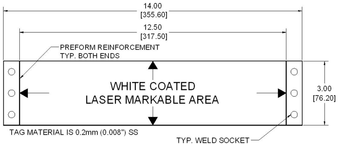
Figure 4 Standard Slab Tag geometry
