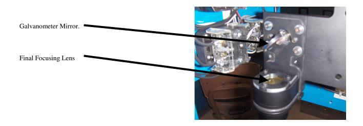
**CAUTION**: <u>DO NOT</u> TOUCH LENS WITH FINGERS OR ANY SUBSTANCE CONTAINING ALCOHOL, OR PERMANENT DAMAGE MAY RESULT.
