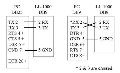
Note: Handshake protocol is XON / XOFF. Communications adapters such as USB to RS232 must support XON / XOFF.
