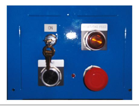
**Reminder -** The marker is not ready for use and will not feed tags until the E-STOP button is returned to the OUT position by pulling red button.
