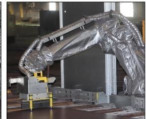
Customized InfoSight **LabelLase® Laser Marking Systems** print barcodes directly onto products.
