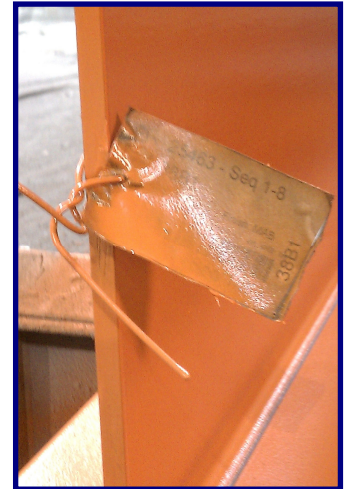
After Shot Blasting and Painting
