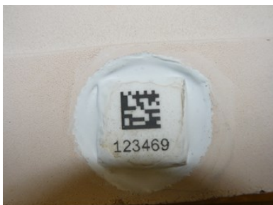
Tile protected in a mold pocket below the surface datum
