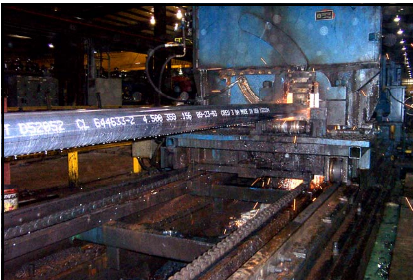
Drop-on demand marker in production, marking on a moving pipe.
