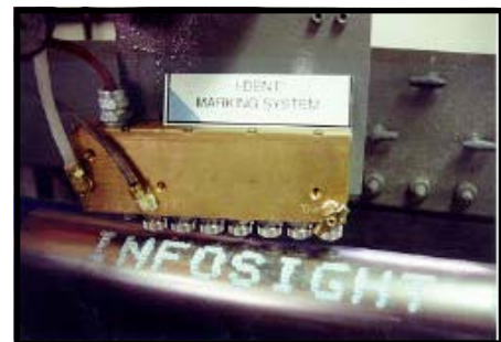
Illustration Shows angle of I-DENT® in relationship to character height.
