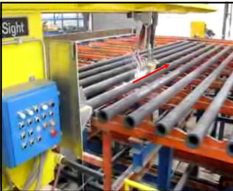
I-Dent® Jib in production, marking on the top of hot static pipe.
